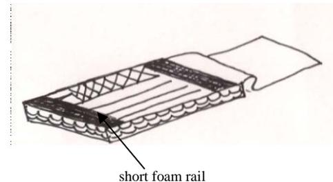
7. Now take the two long foam rails and place them in the cover between the head and foot rails. The side rail is cut out to accommodate the inflator which fits into this cut out.
